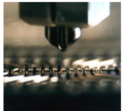
Fig. 2 Miniature gripper WPT/6 used in pull tests on wire bond connections
