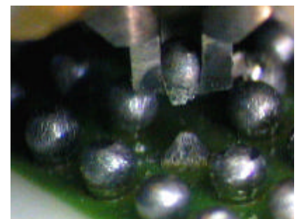
Fig. 2 Pull test on BGA with ball diameter 700\ \mu\text{m}
