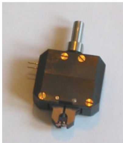
Fig. 1 Ball pull tester BPT/SMD for SMD pull test
